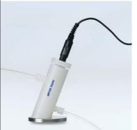
Low conductivity measurement requires special attention. When measuring pure or ultra-pure water there are several sources of potential error such as carbon dioxide from air and temperature inaccuracy. Our digital conductivity cell InLab<sup>®</sup> Trace, with high temperature accuracy and optional flow through cell now provides the perfect solution. Temperature compensation for pure water
